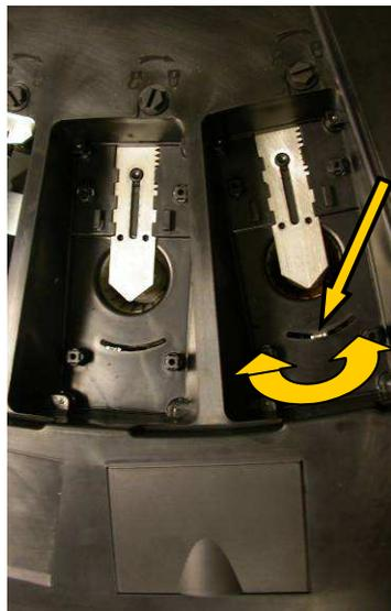
c) Reinsert the hopper and lock it by turning the screw clockwise.
