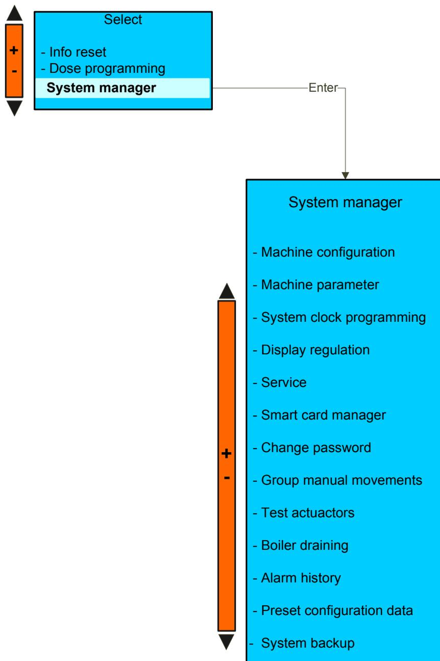
Press the key N°7 (Enter) to confirm entering the desired environment.
