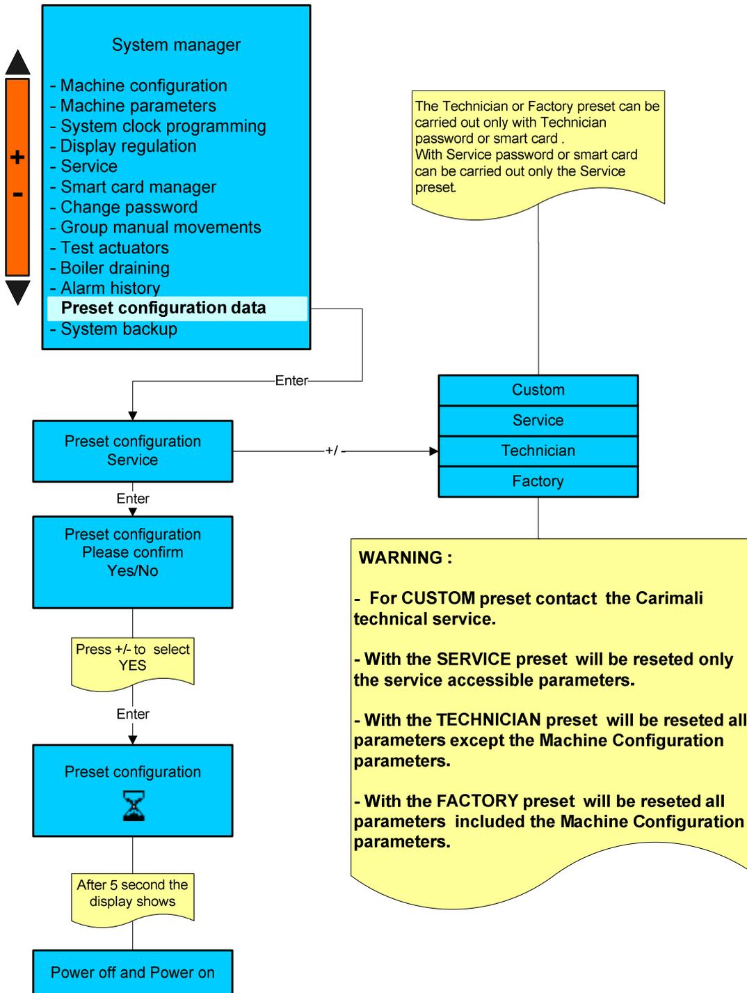
With this function, all the set up values, machine counters and passwords take the default values set up by the manufacturer.
