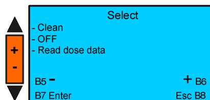
Press the key n°6 ( + ) to select OFF and then press the key n°7 ( Enter ) to confirm.
